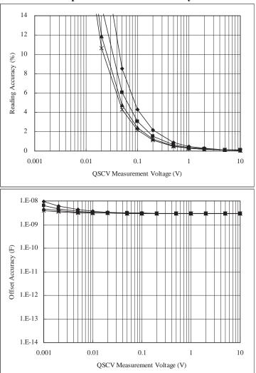
QSCV Operating Mode: Normal Measurement Range: 1  $\mu A$  Output Range: 20 V
