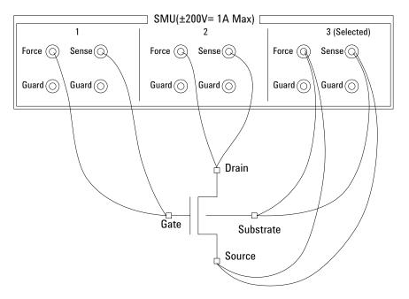
To cancel the effects of the residual resistance, test leads must be connected as close as possible to the DUT.
