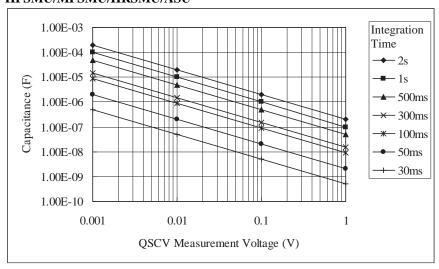
Figure 10-5 Maximum Measurement Value Using 1  $\mu$ A Range: HPSMU/MPSMU/HRSMU/ASU
