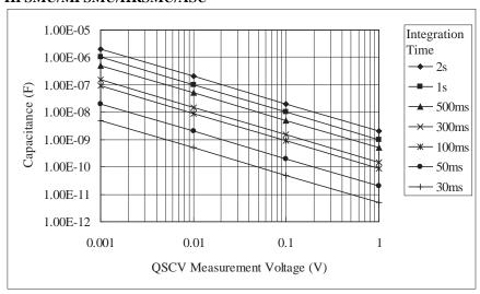
Figure 10-3 Maximum Measurement Value Using 10 nA Range: HPSMU/MPSMU/HRSMU/ASU
