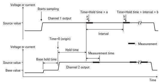
In this figure, *a* and *b* in the formula of *Time* indicate the time from the start of one point measurement to the start of integration by the A/D converter.
