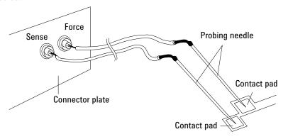
This example uses test leads. To reduce the leakage current, use coaxial cables.
