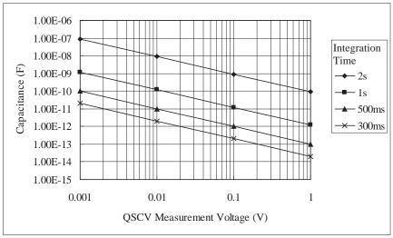
Figure 10-2 Maximum Measurement Value Using 1 nA Range: HPSMU/MPSMU/HRSMU/ASU
