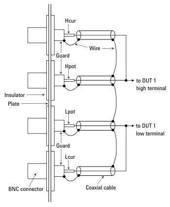
The Hcur/Hpot/Lcur/Lpot lines should be connected to the DUT as shown above.
