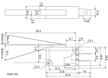
Figure 3-11 Dimensions of the Interlock Switch (Agilent part number 3101-3241)
