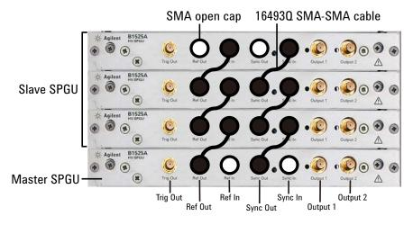
If multiple SPGUs have been installed, connect the SPGUs as shown in Figure 3-7. This connection makes it possible to perform the synchronous output by the multiple SPGU channels. In this figure, the master SPGU is the module which outputs the reference signal and the slave SPGUs are the modules which follow to the reference signal.
