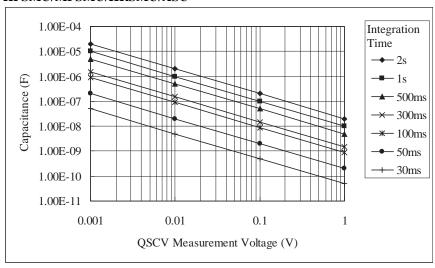
Figure 10-4 Maximum Measurement Value Using 100 nA Range: HPSMU/MPSMU/HRSMU/ASU
