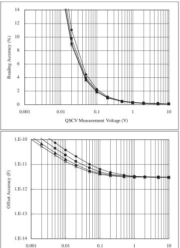
QSCV Operating Mode: Normal Measurement Range: 1 nA Output Range: 20 V
