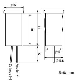
Figure 3-10 Dimensions of the Interlock Switch (Agilent part number 3101-0302)
