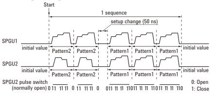
In the example in Figure 7-19, SPGU1 and SPGU2 are used. The channels output Pattern2 twice and Pattern1 three times in one sequence, although the two patterns for SPGU1 are the same.
