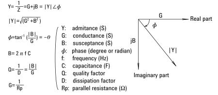
In some case, the reciprocal of impedance (admittance) Y is used. Figure 7-12 shows the vector representation of admittance. As impedance Z, Y contains a real and an imaginary part, and is expressed in rectangular form as conductance G and susceptance B, or in polar form as magnitude of admittance |Y| and phase  $\phi$ .
