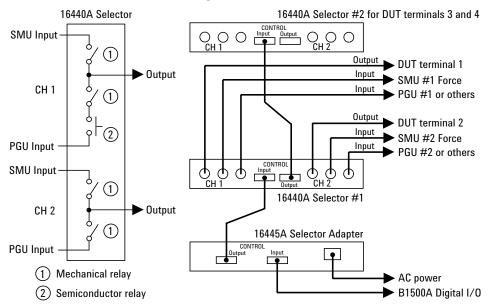
The selector must be connected to the B1500A through the Digital I/O connector and the Agilent 16445A Selector Adapter. Up to two selectors can be used by connecting the selector control cable between the CONTROL Output connector of the first selector and the CONTROL Input connector of the second selector.
