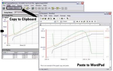
Figure 4-6 shows the list copy and paste example. Click a line of the List Display area on the Data Display window, select Edit > Copy menu, and paste it to Notepad. You will see the result as shown in this example. The data in Notepad is a CSV data (separated by a comma). Save it as a text file and open it by using a spreadsheet software. Each data (comma separated value) will be entered to a separate cell.
