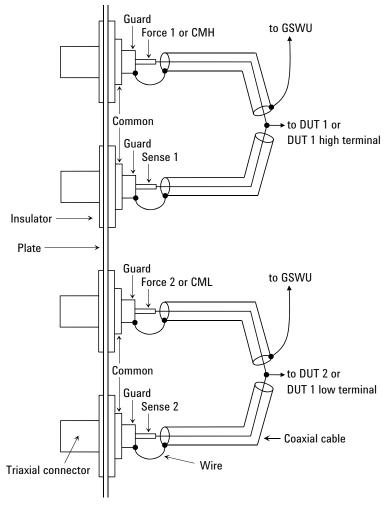
The SCUU should be connected to the DUT by using coaxial cables and wires as shown above. Also the SCUU should be connected to the GSWU inside the shielding box by using a control cable through the 16495K plate.
