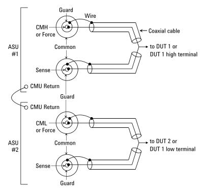
The ASU inputs can be connected to the instruments by using a control cable, a triaxial cable, and two coaxial cables. The cables can be connected to the ASU inside the shielding box through the 16495K plate.
