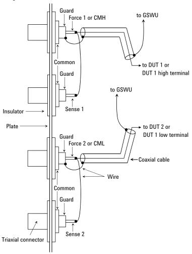
The SCUU should be connected to the DUT by using coaxial cables and wires as shown above. Also the SCUU should be connected to the GSWU inside the shielding box by using a control cable through the 16495K plate.
