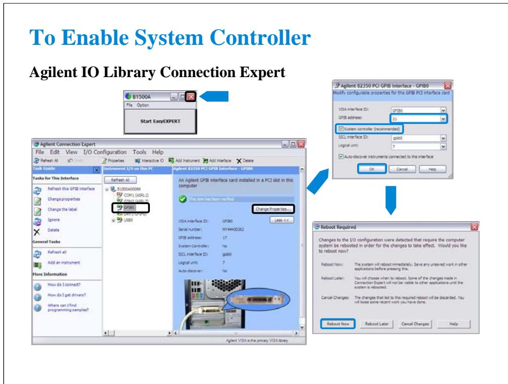
To control external GPIB devices, the B1500A must be set to system controller. Exit the EasyEXPERT, and close the Start EasyEXPERT window. After that, launch the Agilent Connection Expert by clicking Start, All Programs, Agilent IO Library Suite, and Agilent connection Expert.
