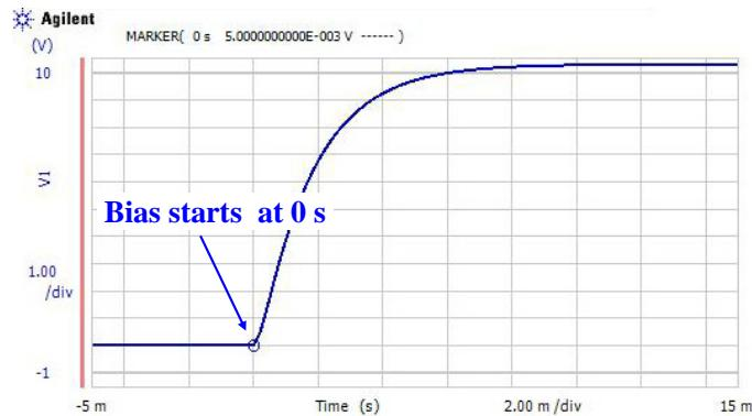
For the sampling measurement, the available hold time value is 0 to 655.35 s, in 10 ms step.
