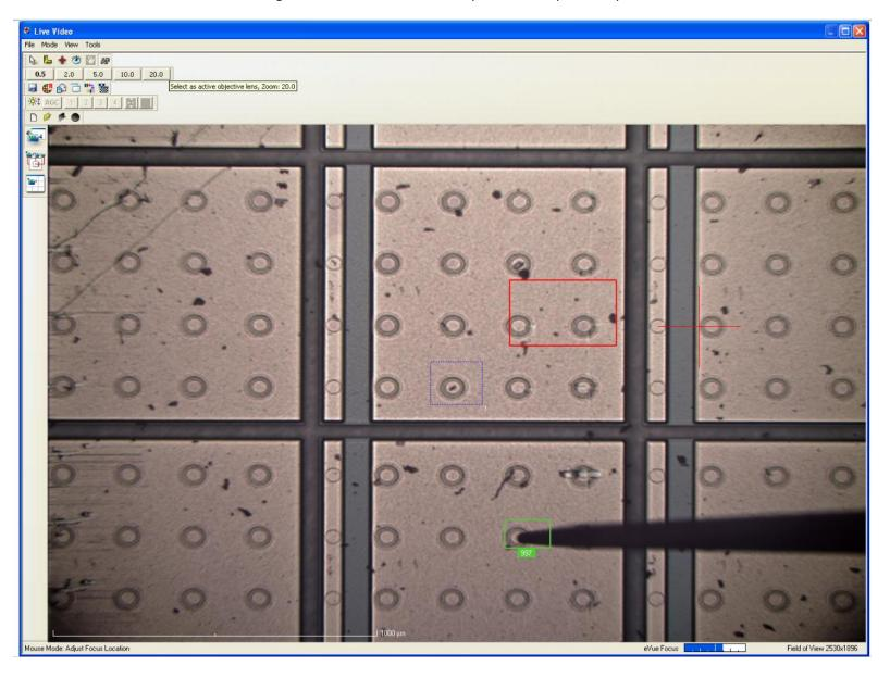
We click on the wafer map to step to another location. The prober goes first to the trained wafer site, acquires the target
