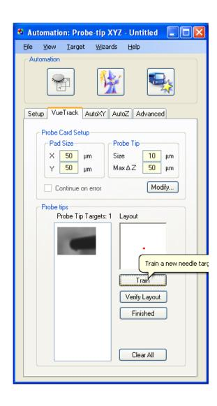
We next train on a wafer target to establish the wafer plane. This should be outside the probe card area.
