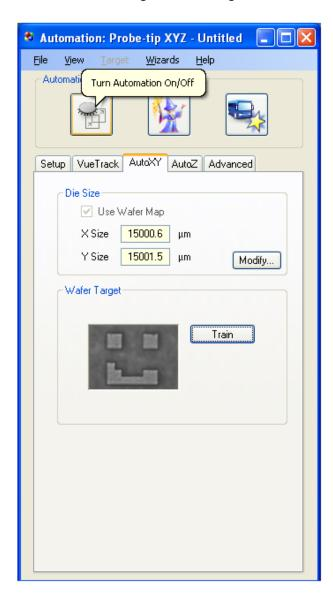
When we turn on Automation the chuck goes to contact at the trained postion with probe to pad.
