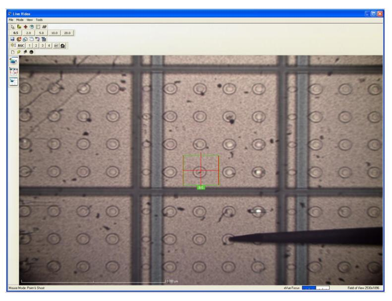
After probe to pad is accomplished, set reference in place.
