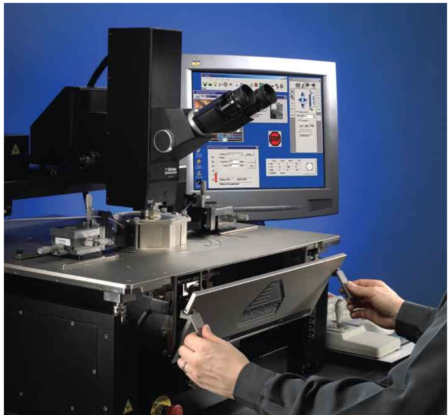
The patented MicroChamber revolutionized wafer probing. It enables over-temperature testing in a light-tight, noise-free, EMI-shielded environment.
